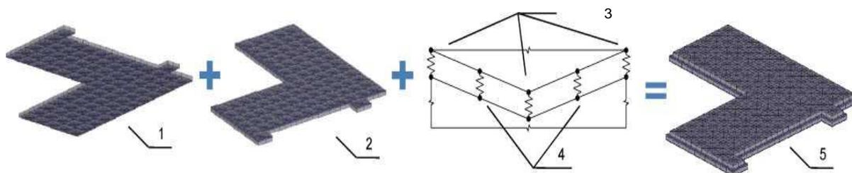
**Figure 4. The scheme of modeling the foundation with a sliding belt:**
