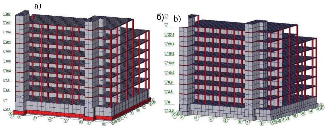
**Figure 5.** Calculation models: a) seismically isolated building; b) non-seismic isolated building
