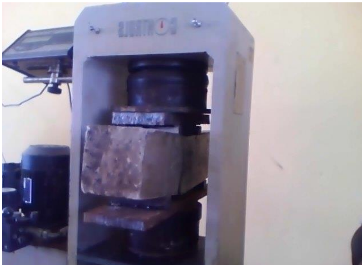
Fig. 3. Testing of Concrete Beams in Flexure.
