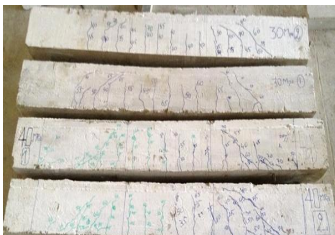
Figure 6. Deformations of reinforced beams.
