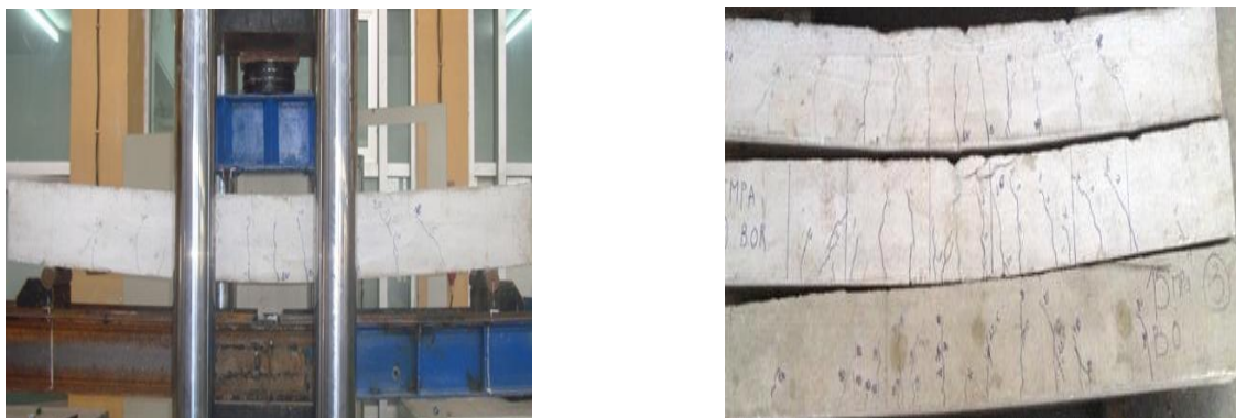
Figure 4. Deformations of unreinforced beams B(OC).
