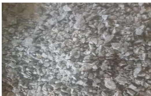
Figure 1: Shredded plastic and aggregates prepared
