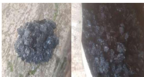
Figure 2: Aggregates coated by plastics
