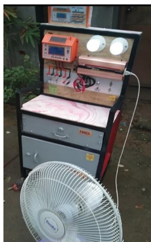
Figure 18. Testing of 2000 Watts Inverter
