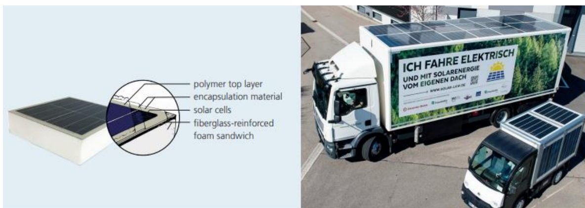
Schematic of a lightweight module for trucks.
