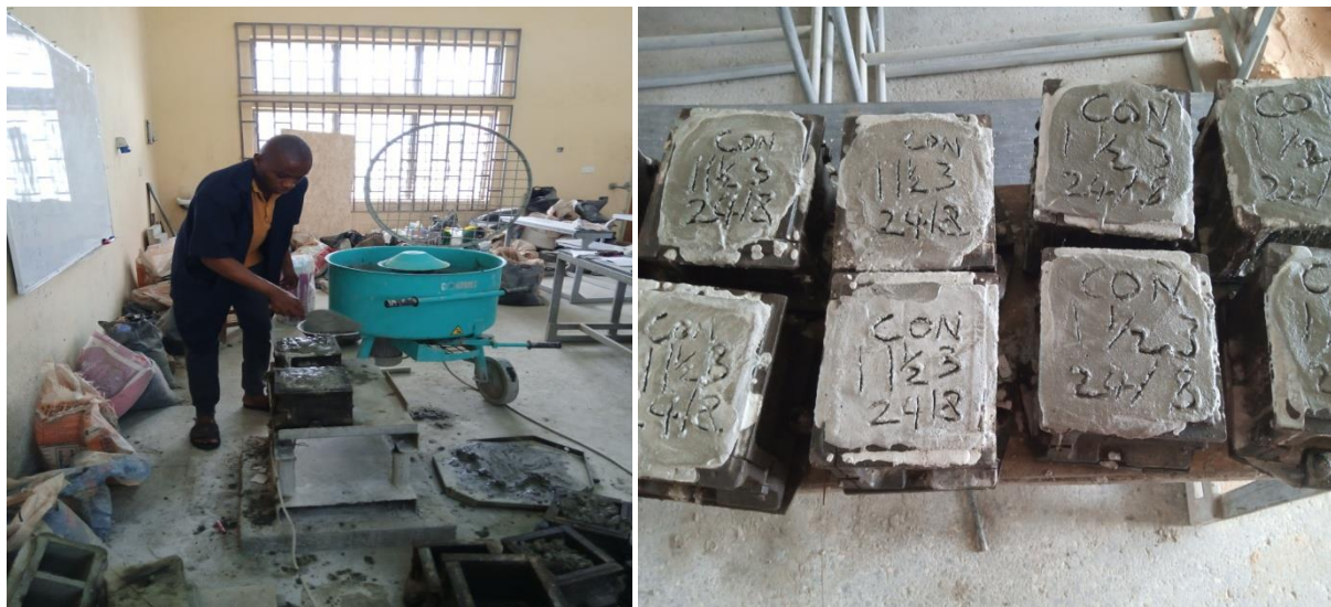
Figure 3.2 Preparation of cubes
