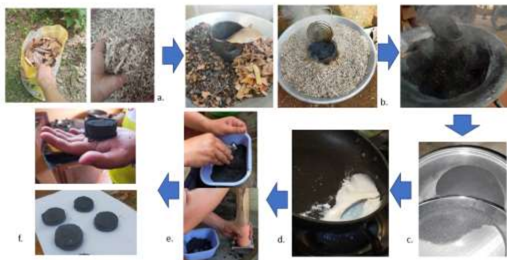
Figure 1. General steps in the development of charcoal briquettes
